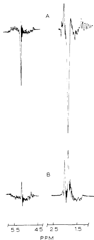
Figure 1. Nmr spectra of ethylene (left) and cyclobutane formed in the reaction of sodium naphthalene with 1,4-diiodobutane. The bottom spectra are the signals obtained after long times. The top spectra were taken a few seconds after the reaction was carried out.
